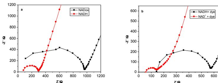
Fig. 1. Impedance spectra presented as Nyquist plots of: a) 500  $\mu\text{M}$  NAD<sup>+</sup> or NADH in 10 mM NaOH; b) NAD<sup>+</sup> or NADH mixed with 50  $\mu\text{M}$  dye D-OH.
