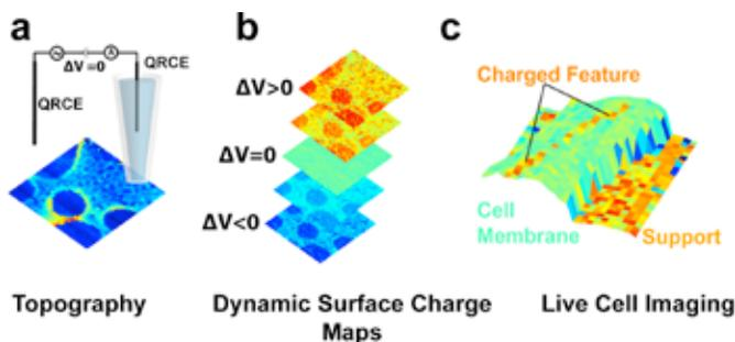
**Figure 1:** Bias Modulated SICM allows for precise probe positioning free from surface charge effects (a) and as a tool for surface charge mapping when a varying bias is applied (b). SICM can be used to simultaneously map the topography and surface charge of viable living cells, identifying surface charge heterogeneities on cell membrane surface, with consequences for understanding the functioning of cells.
