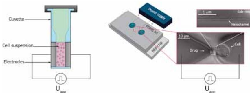
Fig. 1: Classical bulk electroporation (left) and nanochannel electroporation (right).
