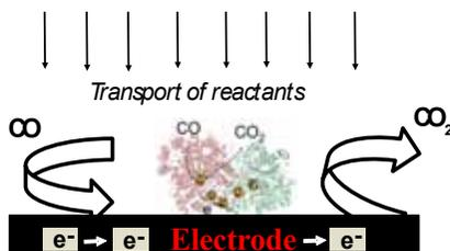
Figure: Schematic representation of a protein film voltammetry technique, CODH is the colorful part deposited at the electrode surface.
