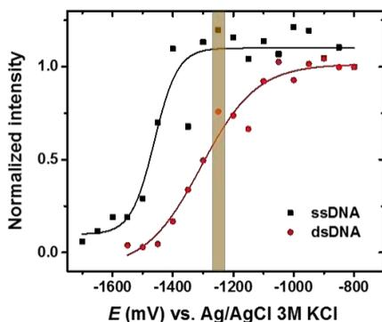
sequences. The analyses were performed on a Au nanovoid modified SERS-active electrode surface using in-situ SERS measurements. Cy3-labeled target DNA was employed as a Raman reporter to observe dehybridization and the corresponding desorption curves. Rapid and uniform surface modifications were achieved via the recently suggested potential-pulse assisted DNA immobilization method [2].
