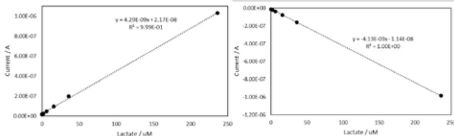
**Fig. 1.** Calibration curve of enzyme modified Pt (left) and Prussian blue modified gold (right) nanoband array electrode towards lactate, operated at 0.55 V and 0.05 V vs Ag/AgCl (respectively).
