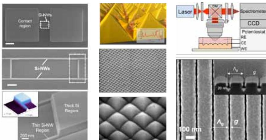
Silicon nanowires (left), gold nanopyramids (middle) and nano-interdigitated electrodes for electrochemical SERS (right)
