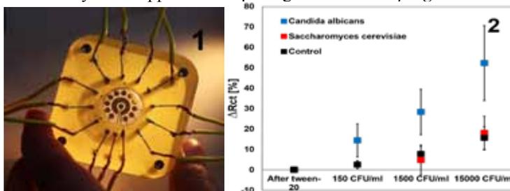
**Figure 1.** Biosensor prototype interfaced with PCB board. **Figure 2.** EIS data presented as relative charge transfer resistance. The biosensor shows high selectivity to *C. albicans*.
