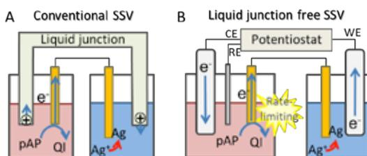
Fig. 1. Schematic illustration showing (A) conventional system and (B) liquid-junction-free system for deposition process of SSV.
