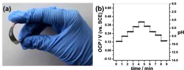
**Fig. 1-** (a) Photographs of hydrogel embedded pH-sensor. (b) OCP of PdO-Pd/Au/PMMA/PET function of time recorded in electrolytes with different pH values.
