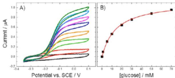
**Figure 1.** A) Cyclic voltammograms for a CDH-modified carbon nanotubes electrode at different glucose concentrations (0-70 mM). B) Plot of the current vs. sugar concentration.
